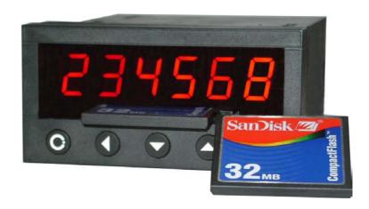
OC7054FC is a 6 digit programmable Datalogger for direct connection to process signals such as 0/4-20mA, 20mV...100V DC or true RMS, Temperature Sensors, Potentiometers and other signal sources. With the keyboard the display can be scaled in required process units. One Set Point Relay is available for controls applications.
